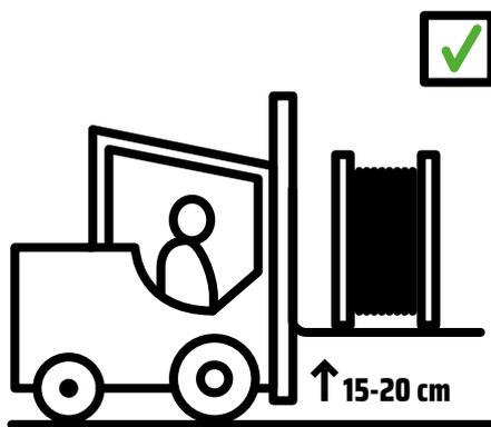
Insufficient lifting height may cause the drum to be dragged on the ground and eventually get damaged or dropped off the forks, especially if the ground surface is uneven. The drums may be placed and stacked on pallets to make it safer and easier to move them.
