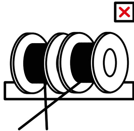
The number of cables to be pulled at the same time is determined by the installation conditions at site: distance to be pulled, open space available for looping the cable at intermediary drawing stations and the routing of cables (number of bends and number of corners).
