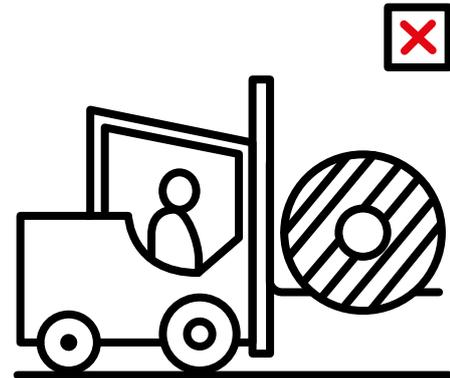
Lifting cable drums with a forklift is only allowed from the "flange side". To avoid damage, never touch the cable or its protective cover with the fork.
