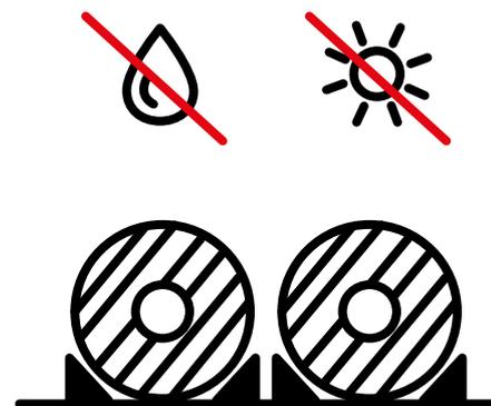
Cables with coloured outer sheaths shall not be stored in direct sunlight to prevent fading. Cables shall be protected against direct sunlight with suitable protective packaging, such as plastic sheeting.
