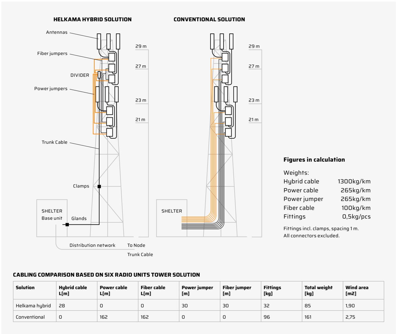
↑ A comparison between the Helkama Hybrid Cable solution and conventional individual power and fiber cabling for six radio and antenna units.
